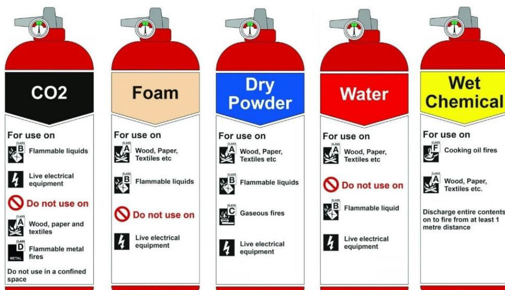
Fig. 9.2.4 Types of Fire Extinguishers
