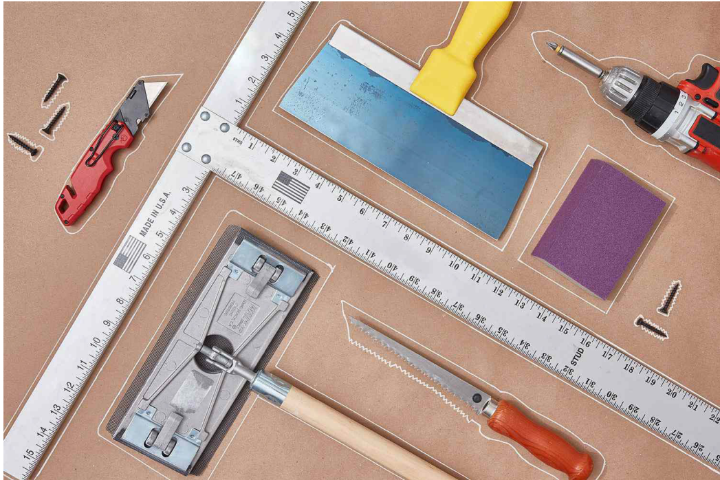
Fig. 6.1.21: Tools and materials for wall panel fixing
