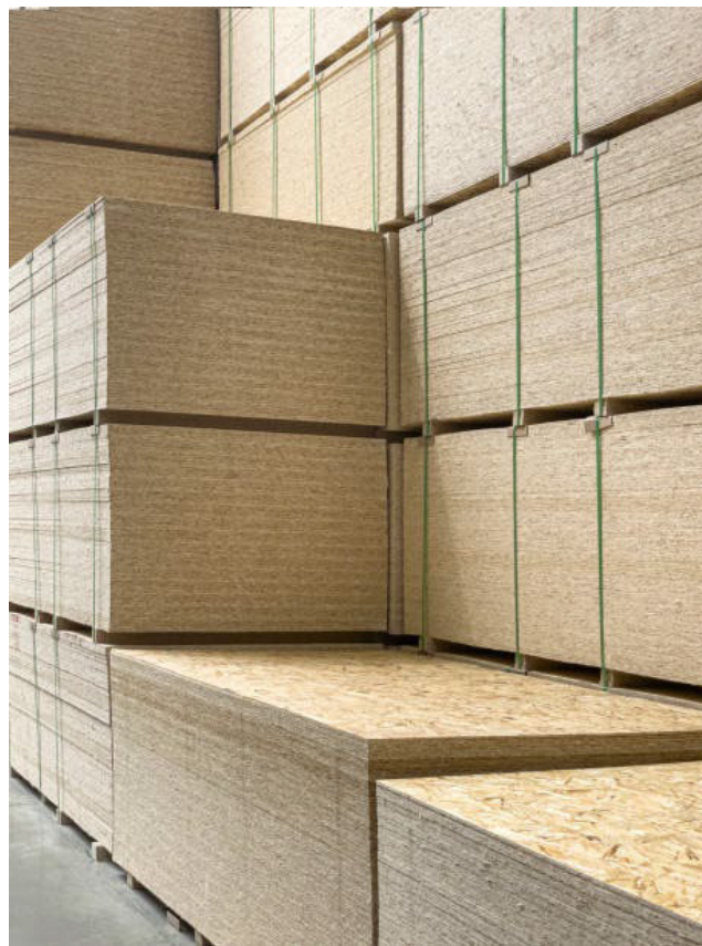
Fig. 3.1.40: Storing and stacking fiberboard
