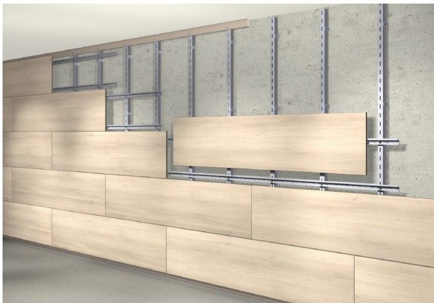
Fig. 6.1.18: Safe and systematic installation of wall panels
