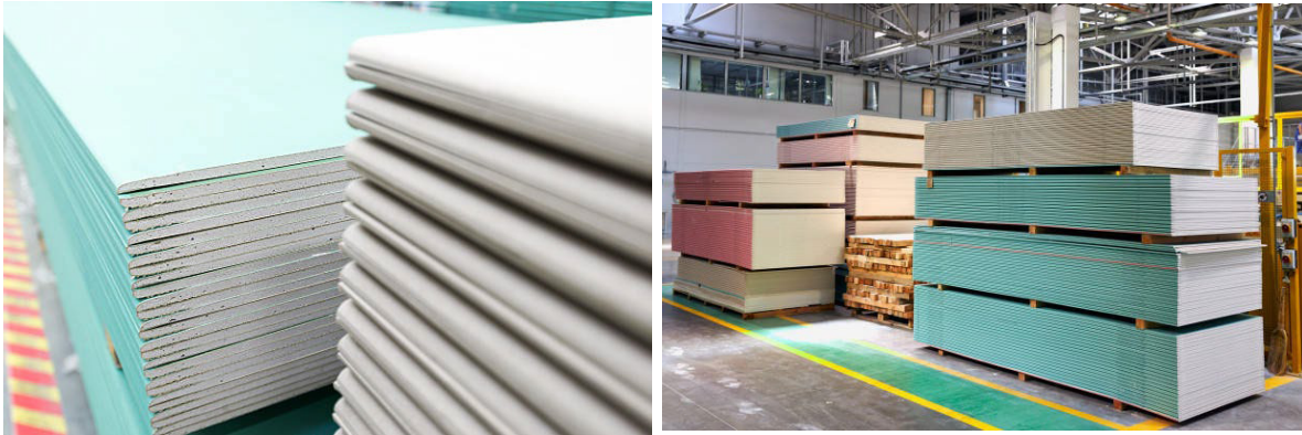
Fig. 3.1.39: Storing and stacking gypsum board
