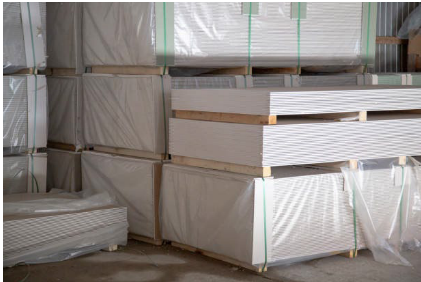
Fig. 3.1.44: Stacking with spacers
