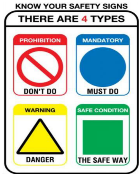
Fig. 9.1.6 Workplace Warning Signs
