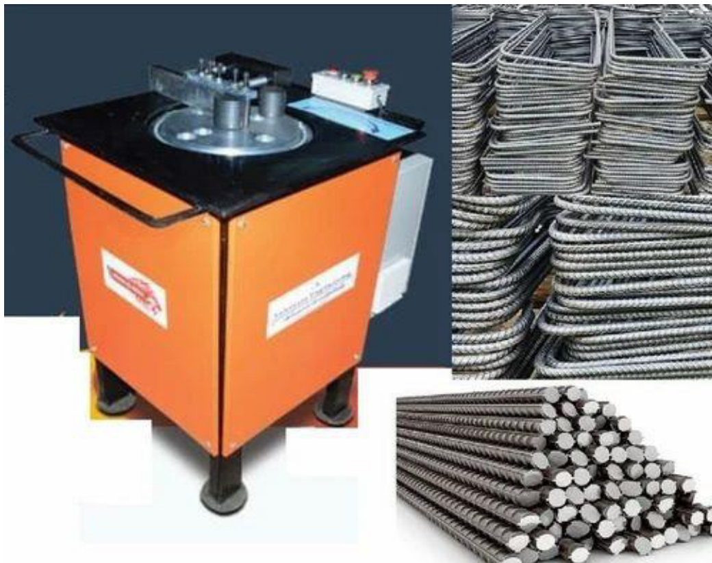
Fig. 4.3.27: Using a motorized bending machine
