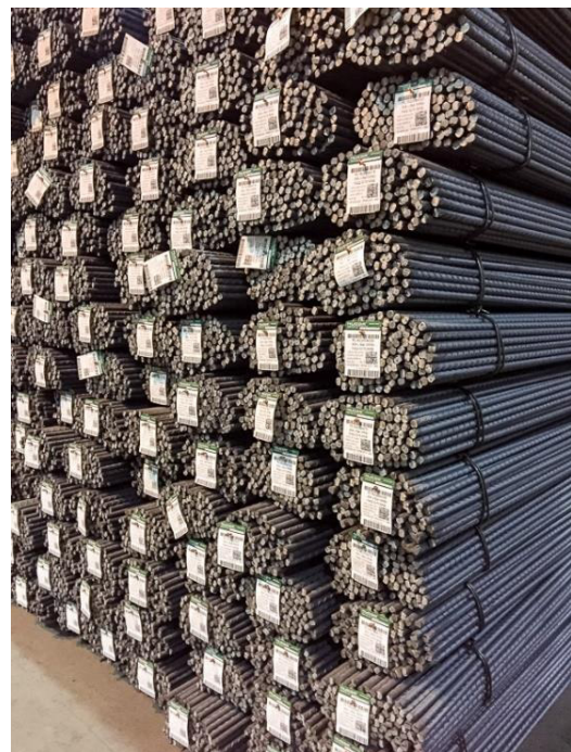
Fig. 4.4.6: Tagging of rebar
