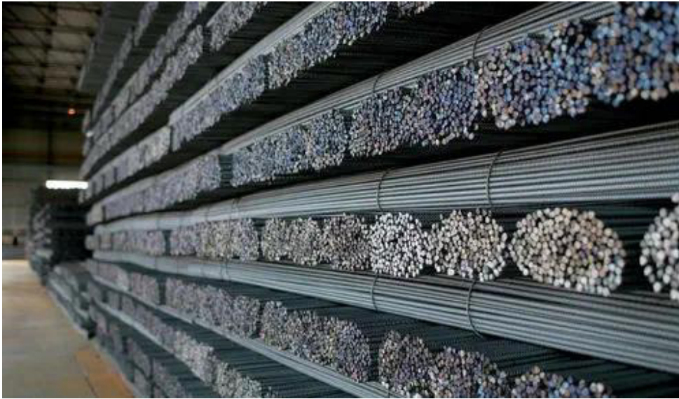
Fig. 4.4.4: Storage and stacking of rebar
