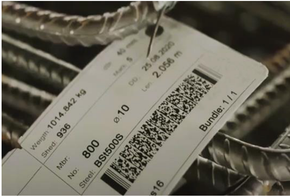
Fig. 4.4.8: Tagging of rebars
