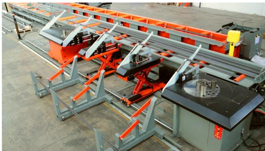
Fig. 4.3.16: Automatic reinforcement cutting and bending machine
