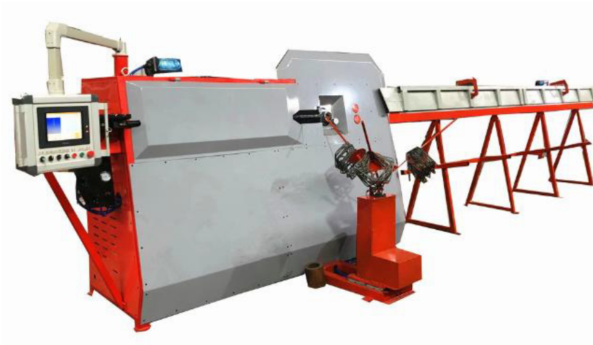
Fig. 4.3.17: CNC reinforcement cutting and bending machine
