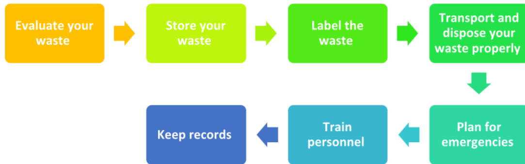
Fig. 8.2.5 Waste collection and disposal process
